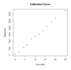
If we wish to add a line to the plot to illustrate the linear regression between the x's and y's, we create a model object, plot the (x,y) pairs, and then plot the model object using the " $Im(y\sim x)$ " and "abline()" functions
