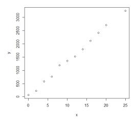
We can label the plot by adding in more commands: plot(x,y, xlab="Conc,mg/L", ylab="Response", main="Calibration Curve") and hence we get:
