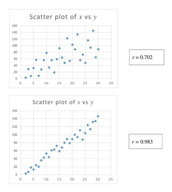
In plotting an instrumental calibration curve between concentrations of standard solutions versus instrument responses, a high Pearson correlation coefficient of >0.99 is normally desired.
