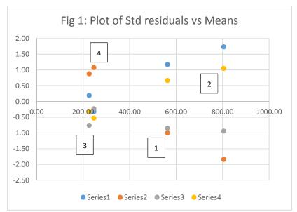
The Figure 1 indicates the most common pattern of non-constant variance in which the error variance increases as the mean response increases, with its plot showing a megaphone in shape.
